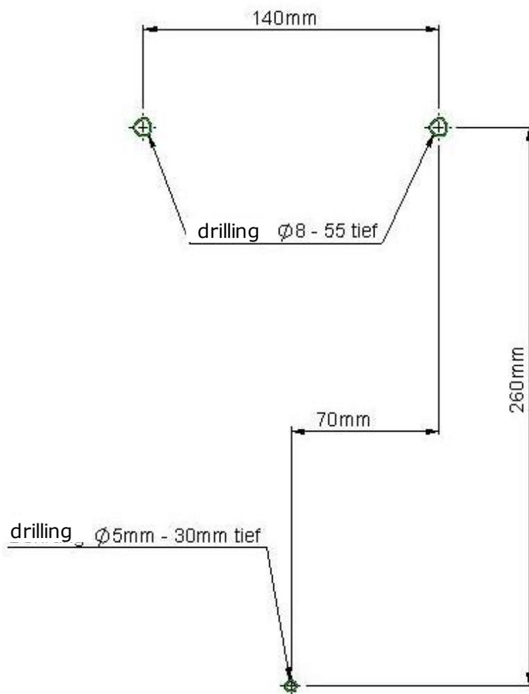
Secure the enclosed screw anchors as shown in Figure 1. Screw the 6x50 screws into the two upper holes; keep a distance of 6-7 mm to the wall! (Figure 2)
