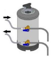
Depressurisation and salt-refilling mode (valve "C" and "D" to the right)
