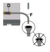
The outflowing water during regeneration must be directed to a drain.
