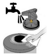
Check the seal on the lid and the top part of the Wasi-Clean for any residues of salt or resin, clean if necessary and then fit the lid and screw it tight.
