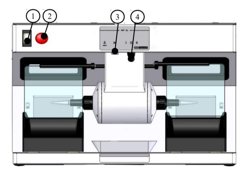
(1) Main / Protection switch: The device is powered.
