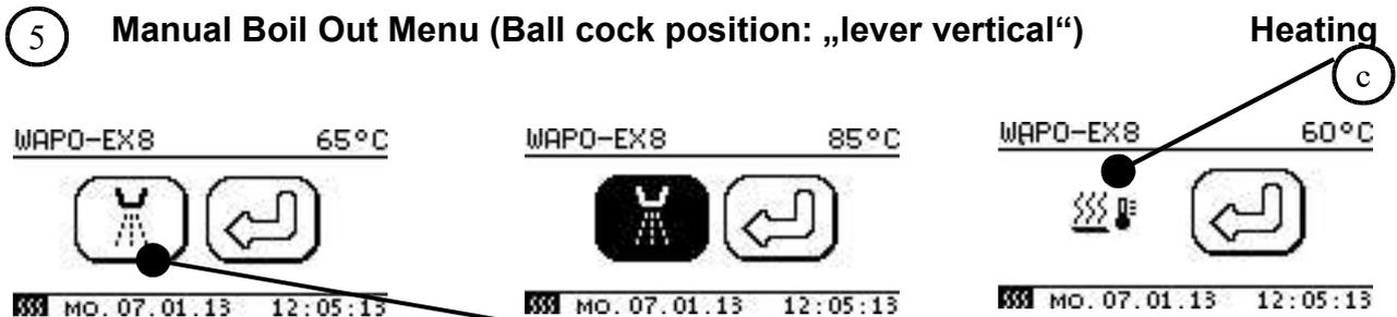
The manual boil out process is initiated by touching the **boil out symbol**.
