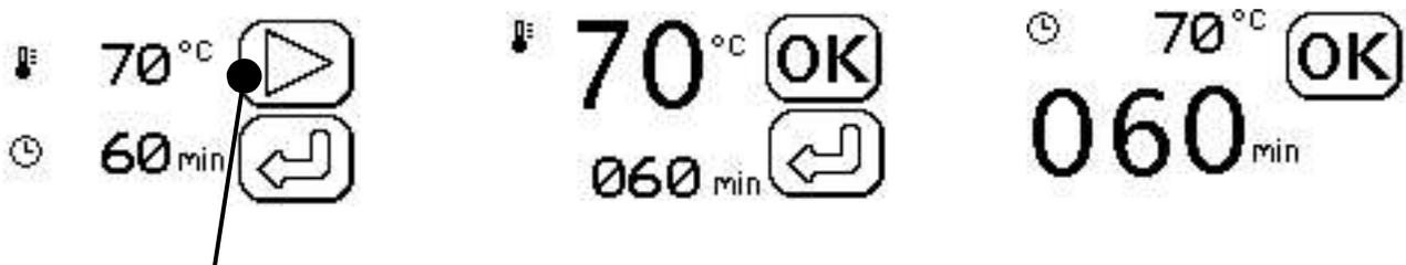
Press the Start button to start the program. Interrupt or stop the program by using the Stop/ Interrupt button.
